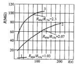
1-Before drying,15 degree Celsius; 2-When the end of drying, 73.5 degree Celsius 3-After running 72h, and cooled to 27 degree Celsius
