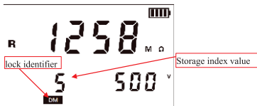
Figure 12-1 Lock and save display
