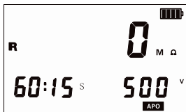
Figure 9-1 Absorption ratio mode 15 second mode
