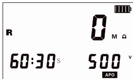
Figure 9-2 Absorption ratio mode 30 seconds mode
