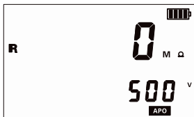
Figure 9-4 Insulation resistance measurement mode
