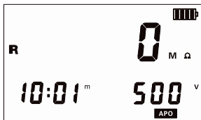
Figure 9-3 Polarization index mode
