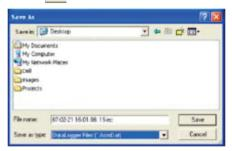
2. Name the file and save it with the default extension. The file will be saved with the ".record" extension to be reopened in the HT Datalogger software program and also as a ".xls"file to be opened in spreadsheet program or other word processing program. To open an existing data file for viewing on the data graph window, click on the limit icon. When prompted, select a .record file saved earlier.
